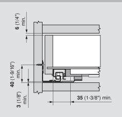
NOTE: TANDEM runners will sit 3 (1/8") higher when using the lateral stabilizer in bottom mount applications and may have to be raised for some bottom mount drawer applications using SERVO-DRIVE
